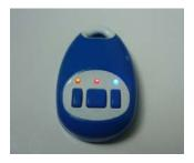
Switch on the unit outdoors. Three LEDs will light at the same time during the tracker starting.
